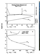
Figure 1:Depth profiles of O<sub>2</sub> and CH<sub>4</sub> concentrations in a) the Notigi Reservoir (northerm Manitoba), and in b) Lake 227 at the Experimental Lakes Area, northwestern Ontario. The dashed horizontal lines represent the depth of the mixed layer.
